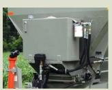
Optional self contained PTO Hydraulic option with oversized oil tank.
