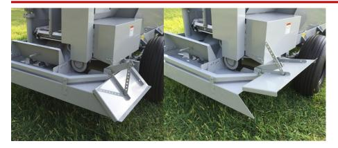
3. With its improved nine-position side limiting deflectors, Stoltzfus orchard/vineyard spreaders can narrow the spread width to as little as six feet, ensuring that materials are spread at the base of the plants.
