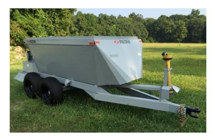
4. Redesigned front and side shields gently direct limbs away from the Stoltzfus orchard/vineyard spreader support structure, protecting tree branches and vines against damage.
