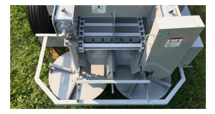
2. A new bolt-on application for Stoltzfus orchard/vineyard spreaders allows quick and easy conversion to general field use.
