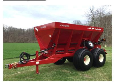
Stoltzfus Spreaders CU100 10-ton Redhawk<sup>™</sup> ground-driven spreader has a heavy duty walking beam, oversized 21.5L tires and a patented dual contact press wheel. Its multi-use applications include packed damp lime, litter and fertilizer.
