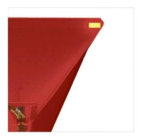
**Steep Side Slopes:** Steep 53-degree side slopes on the RC-8010 spreader ensure steady flows of lime, while 45-degree sides on the RC-8012 provide high capacities of fertilizer.
