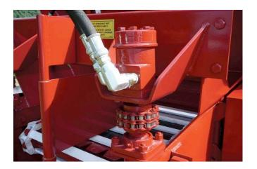
Top-Driven Spinners: Dual hydraulic spinners are top driven, reducing chemical exposure to their motors and safely isolating them from bending forces caused by material pounding on spinner disks.
