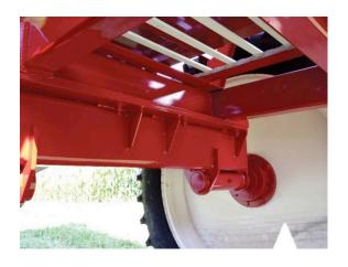
Easy Swap Axle: RC-8010 and RC-8012 come with a choice of wheel tracks between 72 and 120 inches, with bolted-on Easy Swap™ axles that can be changed out for wheel spaces suitable to future row crop requirements. This industry-first feature gives growers an inexpensive way to accommodate future crop spacing needs without having to buy a new spreader.
