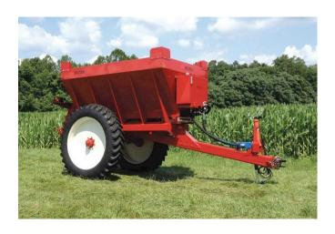
Stoltzfus RC-8010 Spreader: The Stoltzfus RC-8010 Spreader is 10 feet long, weighs 5,800 pounds, has a hopper volume of 177 cubic feet and distributes up to 7,000 pounds of lime per acre. It also handles fertilizer, compost, chicken litter, sand, gypsum and other bulk materials.
