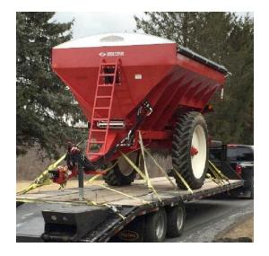
**Stoltzfus RC-8012 Spreader:** Ready to ship, the Stoltzfus RC-8012 spreads all types of fertilizers with application rates as low as 125 pounds per acre. It also distributes lime and other bulk materials, including those spread by the RC-8010. The RC-8012 weighs 6,300 pounds and has a 12-foot-long hopper with 332-cubic-foot capacity.
