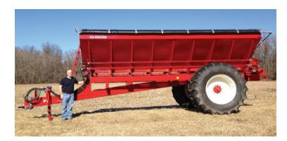
Bernard Hershberger, owner of Stoltzfus Spreaders and grandnephew of C. U., with recently introduced Stoltzfus RC-1520 high-capacity lime and fertilizer spreader with welded unibody construction and axle settings adjustable up to 152 inches, widest on the market.
