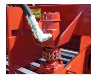
**Top-Driven Spinners:** Dualhydraulic spinners are top-driven, reducing chemical exposure to their motors and safely isolating them from bending forces caused by material pounding on spinner disks.
