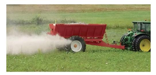
**RC-1516 Lime Spreader**: The Stoltzfus RC-1516 Spreader hopper is 16 feet long, weighs 9,100 pounds, has a volume of 300 cubic feet and distributes up to 7,000 pounds of lime per acre. It also spreads fertilizer, compost, poultry litter, sand and gypsum. The RC-1516 and the RC-1520 spreaders broadcast spread patterns up to 80 feet and are the only spreaders with fully welded unibody construction.
