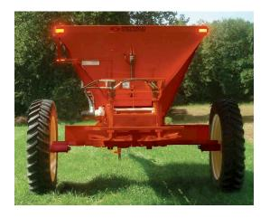
Widest Adjustable Wheel Tracks: New Stoltzfus 15-ton-capacity spreaders come with the industry's widest adjustable wheel tracks, allowing flexible axle settings in two-inch increments up to 152 inches, surpassing other high-capacity spreaders on the market by at least 30 inches.
