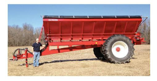
**RC-1520 Fertilizer Spreader:** The Stoltzfus RC-1520 Spreader weighs 12,200 pounds, has a 20-foot-long hopper with 510-cubic-foot capacity and spreads fertilizer from 125 pounds to 4,000 pounds per acre.
