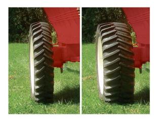
Choice Of Tires: Buyers can select narrow row crop tires for in-row applications or wider flotation tires for low compaction in open field operations.
