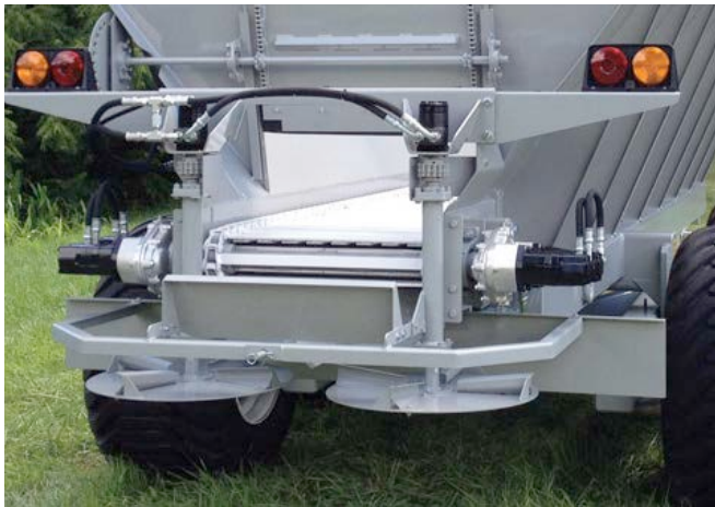
Two top-driven, 24-inch spinner drives are isolated from corrosive chemicals and the shock of material pounding on disks
