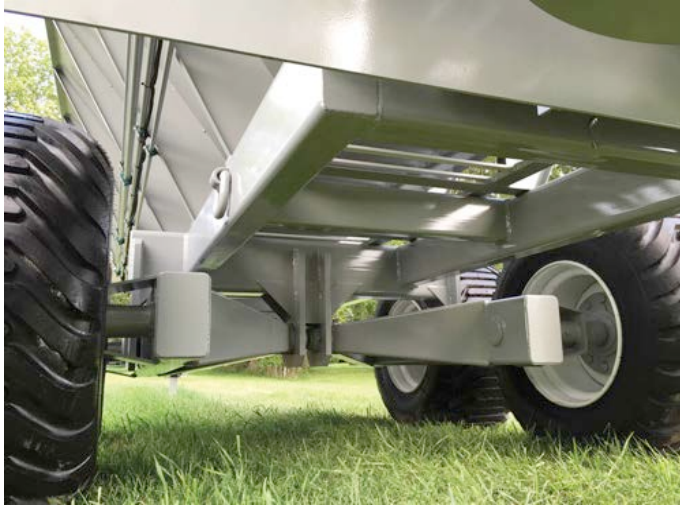
A fully welded walking beam suspension with structural steel tubular frame handles stresses from 20-ton loads with ease, whether on flat ground or rolling hills.
